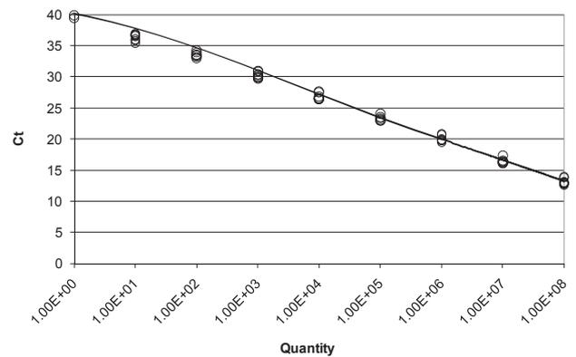
FIG. 2—Consistency among different quantitative PCR (qPCR) standard lots. Four different lots of synthetic standard were prepared and subjected to qPCR in duplicate, and a standard curve plot consisting of all lots was generated ( $R^2 = 0.9960$ , efficiency = 98.6%). The ranges for individual standards varied from 1.2 Ct ( $10^7$  copies) to 1.5 Ct ( $10^1$  copies). Standard quantities of  $10^0$  represent the Y-intercepts of the trend lines for each of the four standards.
