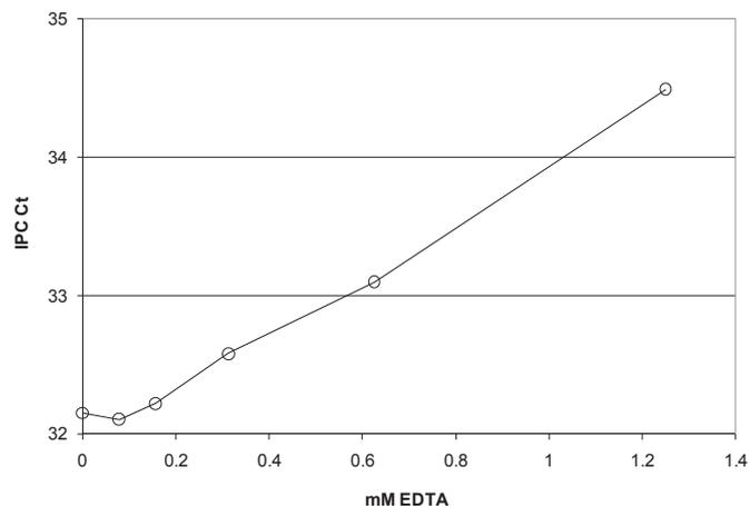
FIG. 4—Inhibition of internal positive control (IPC) signal by EDTA. A stock EDTA solution was twofold serially diluted and added to wells in quadruplicate to yield final concentrations ranging from 10 to 0.078 mM. Average cycle threshold (Ct) values are shown, and Ct values for final EDTA concentrations  $\geq 2.5$  mM were undetermined.
